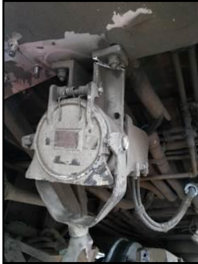
Gambar 14. Adaptor coupler electric rusak
