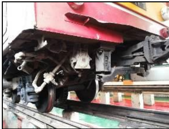
Gambar 6. Cow hanger rusak parah
