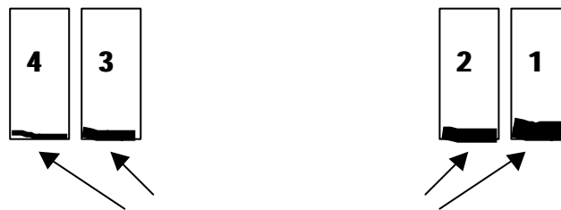
Figure 3. The tire damage on the main wheel surfaces (worn spots on each main wheel) - front view
