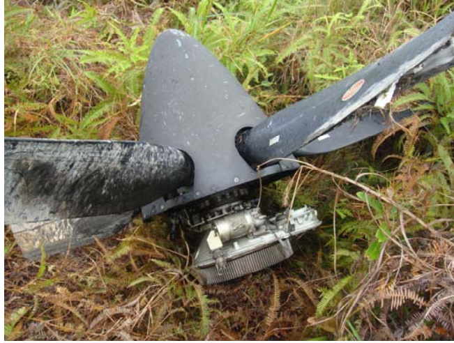
Figure 7: Right propeller and section of the propeller gear box
