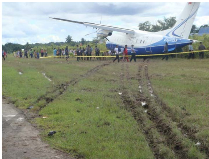
Figure 2: Wheel marks on the muddy runway shoulder
