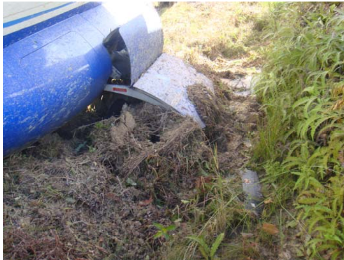
Figure 10: Propeller hit an earth hump (underneath the front of RH gear)
