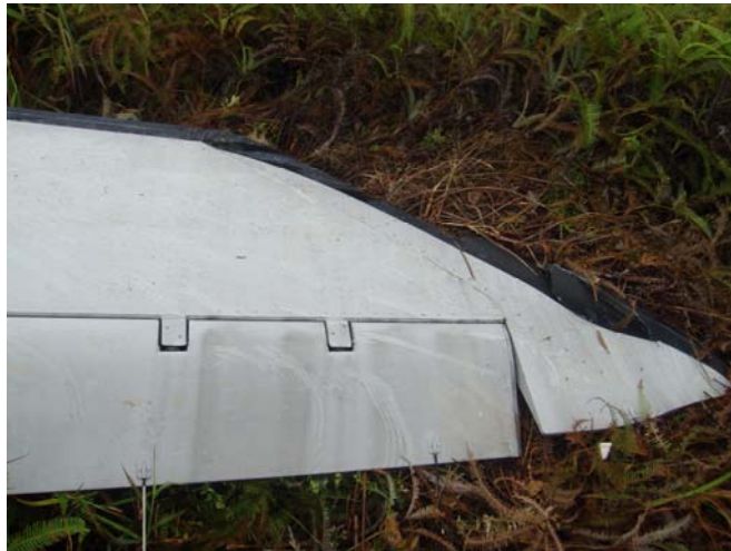
Figure 8: Right wing tip damage, no wrinkles on wing
