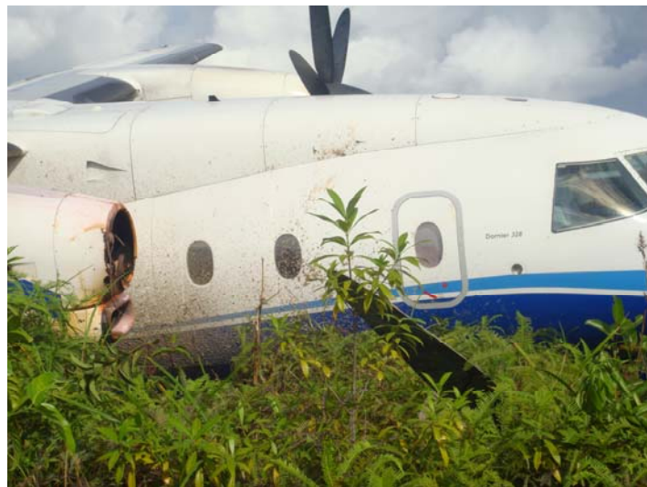
Figure 6: Propeller position 4.5 meters away from the engine
