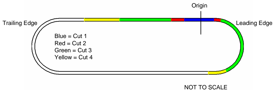
Figure 1. Cross section through spar showing crack positions.
