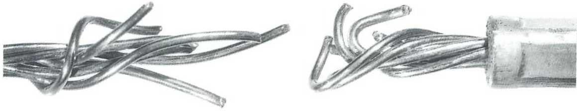
Fig 3 Bent wires on both sides of cable break
