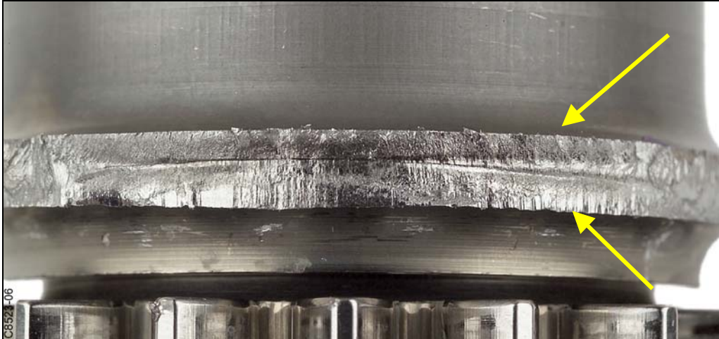
Photo C9: Fractographic examination of the fracture surface on Sector 5, indicating the crack origin regions at the end of the fillet radii.
