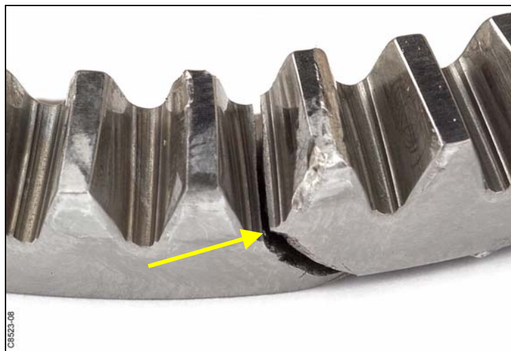
Photo C6: Crack initiation between Sectors 1 and 2 consistent with maximum stress on starting
