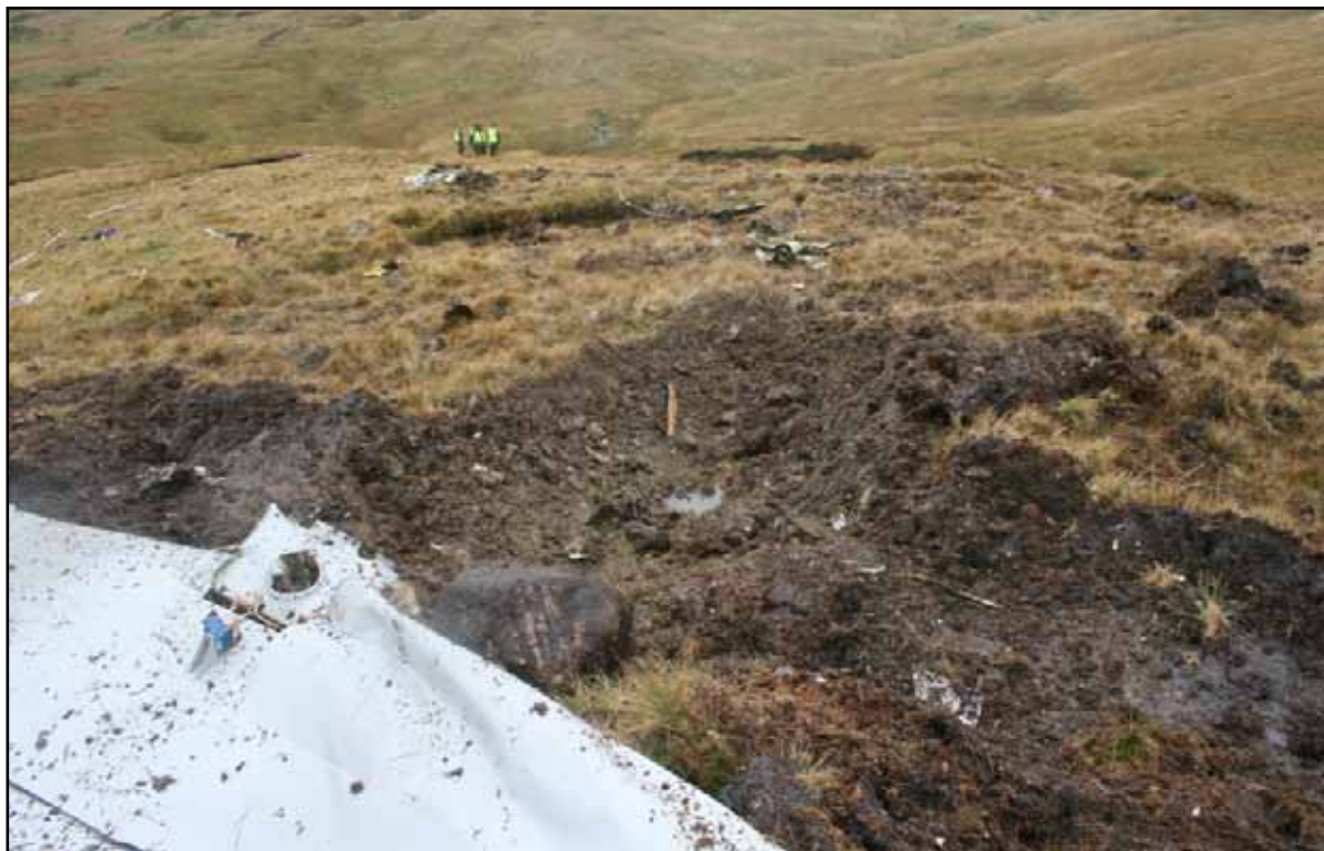
Photo No. 1: Tailplane, impact crater and initial debris trail (in the direction of travel)
