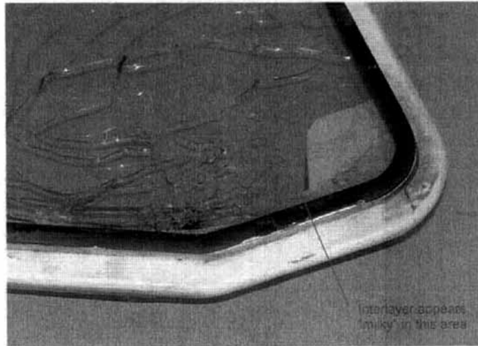
Fig 2 Close-up of failure origin
