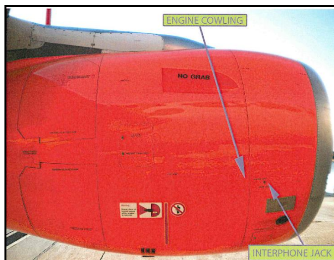
Foto 3: service interphone e fan cowl door.
