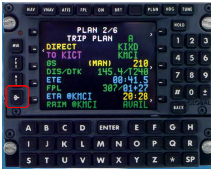
Foto 7: Flight Management System GNS-Xls.
