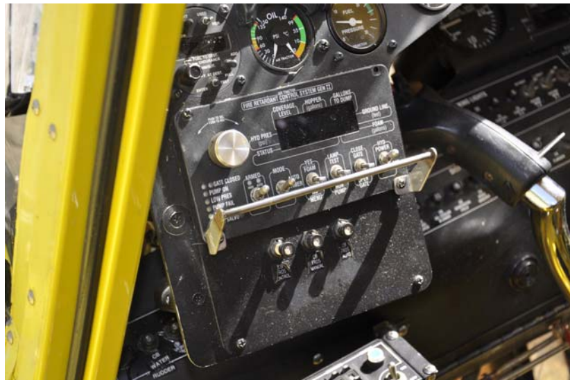
Foto 18: Fire Retardant Delivery System (FRDS).
