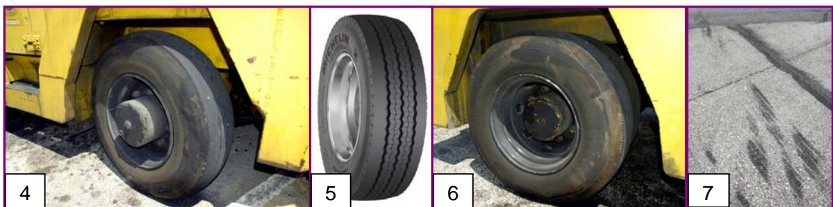
Fig N°4–right front tire. Fig N°5–original tire. Fig N°6–right rear tire. Fig N°7–ground brands.
