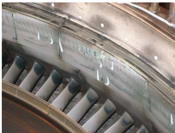
Fig 7 – Severe burning to a coule of HPT Shrouds (removal cause)
