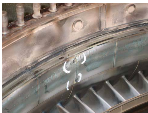
Fig 8 – Burning to more HPT Shrouds. 100% are likely to scrap.
