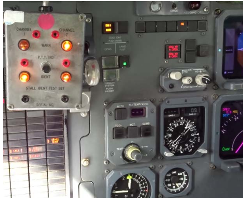
Figure 13. Annunciations on the instrument panel and test equipment, at stick push.
