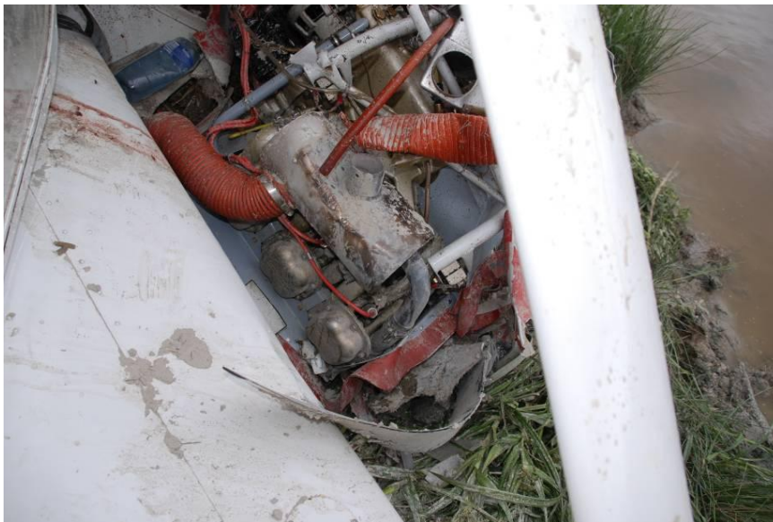
Fig. 5. Engine and propeller blade.
