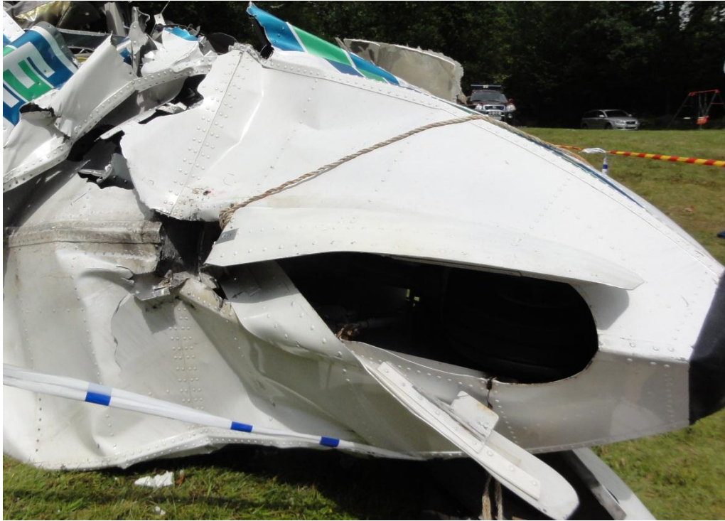
Fig. 5. The underside of the nose, with soft indentations.
