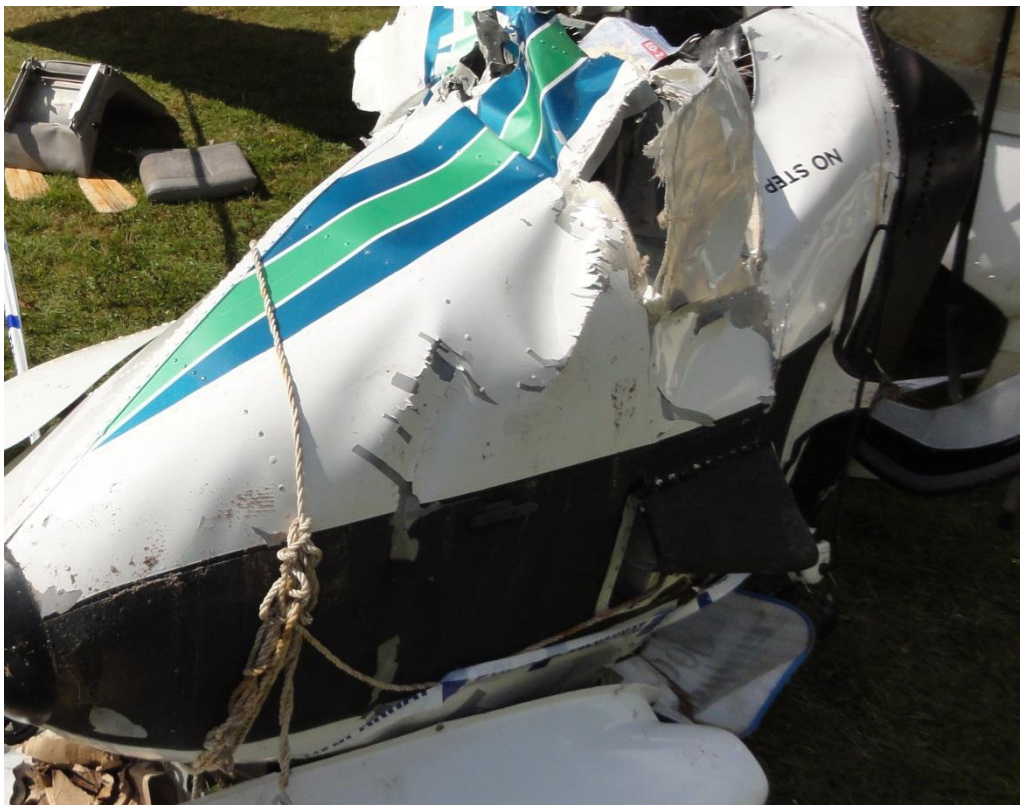
Fig. 6. The topside of the nose had compression folding.
