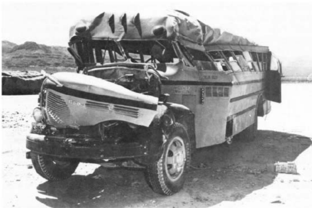
Figure 5.87b. Typical public bus damaged by a nuclear explosion, Nevada Test Site; this bus, like the one in the left background, was overturned, coming to rest as shown after a displacement of 50 feet.
